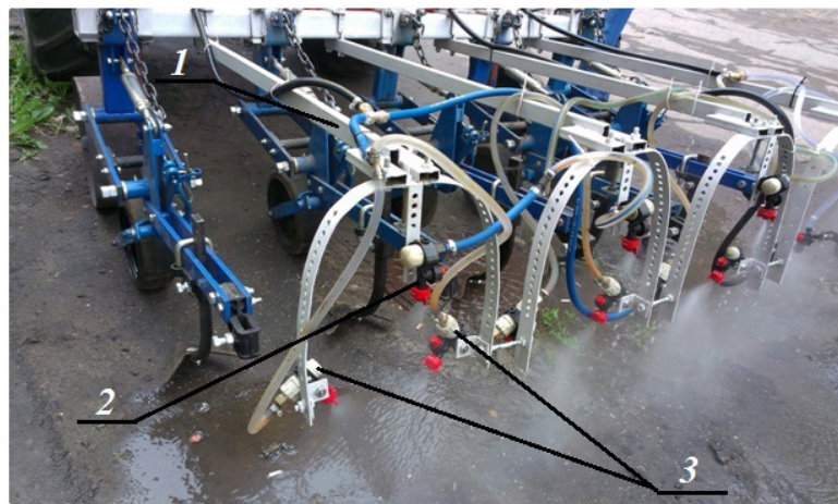
Figure 1. Experimental device for application of growth regulators and herbicides. Notes: 1 — cultivator; 2 — top disperser; 3 — side dispersers
